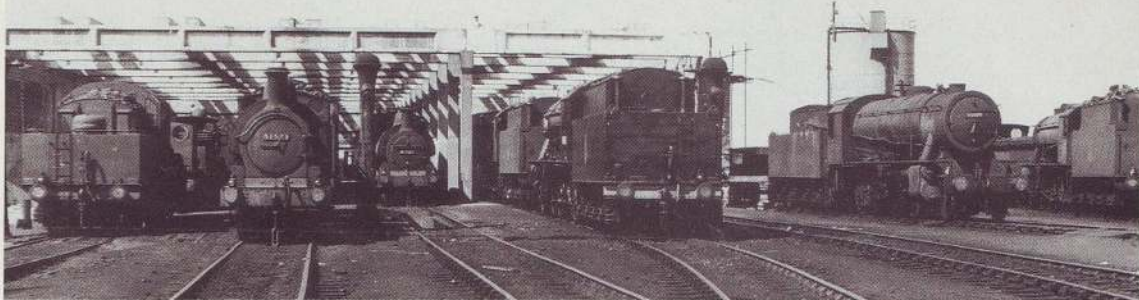
A view of Goole Shed in 1955, with an interesting mixture of locomotives including (from left) an Ivatt 2MT 2-6-0, two of Aspinal's 0-6-0STs rebuilt from Barton Wright 0-6-0s, Nos. 51521 and 51323 and at least four WD 2-8-0s including No. 90609. Photo: K. Hoole/N. E. Stead Collection.
