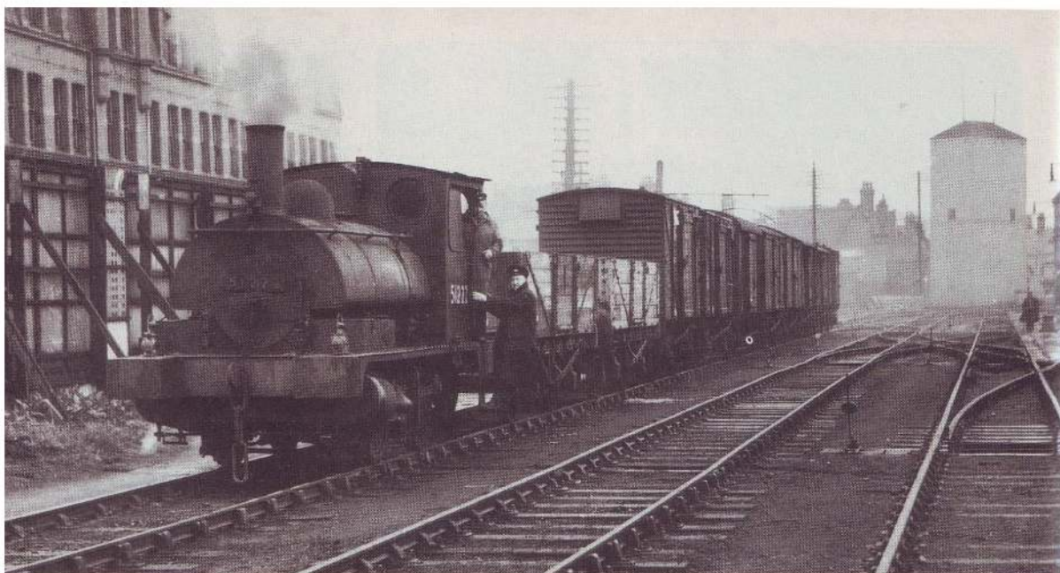
A 'Pug' on the prowl: Aspinal 0-4-0ST No. 51222, formerly of the Lancashire & Yorkshire Railway, busies itself on a damp morning in Goole during the 1950s. Photo: G. M. Staddon/N. E. Stead Collection.
