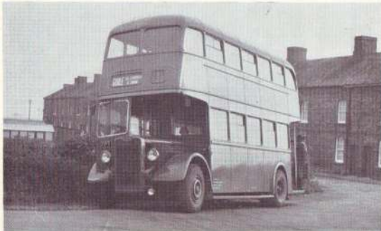
Reliance (R. Store) Ltd. are the present owners of FPT-207, an ex-Sunderland District wartime Guy Arab II fitted with post-war Roe body and "low" Arab III-type radiator, seen on the Doncaster side of Rawcliffe Bridge.
