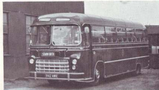
A Bedford SBI with Yeates Pegasus 44-seat dual purpose bodywork incorporating the Yeates conversion giving an entrance position ahead of the front axle. Reliance's 942 AWR is representative of the type of vehicle used on the bridge between Sundays and Fridays, together with one double-decker on the other turn.
