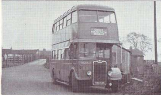
Blue Line's HWU 438, a Guy Arab III with Guy-built body, on the Goole side of Rawcliffe Bridge. A 5-ton weight limit is enforced on this bridge, visible in the background, giving rise to the complex working arrangements described in the accompanying article.
