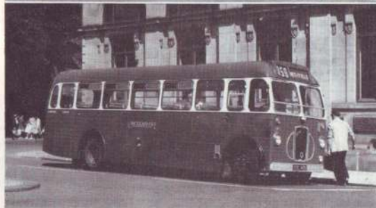
Lincolnshire 2487 (OVL 496), a Bristol 3CALK with E.C.W. body, on the Goole town service.
