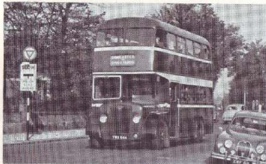
Guy Arab IV YWX 644 is one of the vehicles regularly used by Premier (Harold Wilson Ltd.) of Stainforth, on the Doncaster to Thorne and Moor-ends route. The Roe forward-entrance body is built to 27ft 6in by 8ft dimensions. [All photos: M. Fowler]
