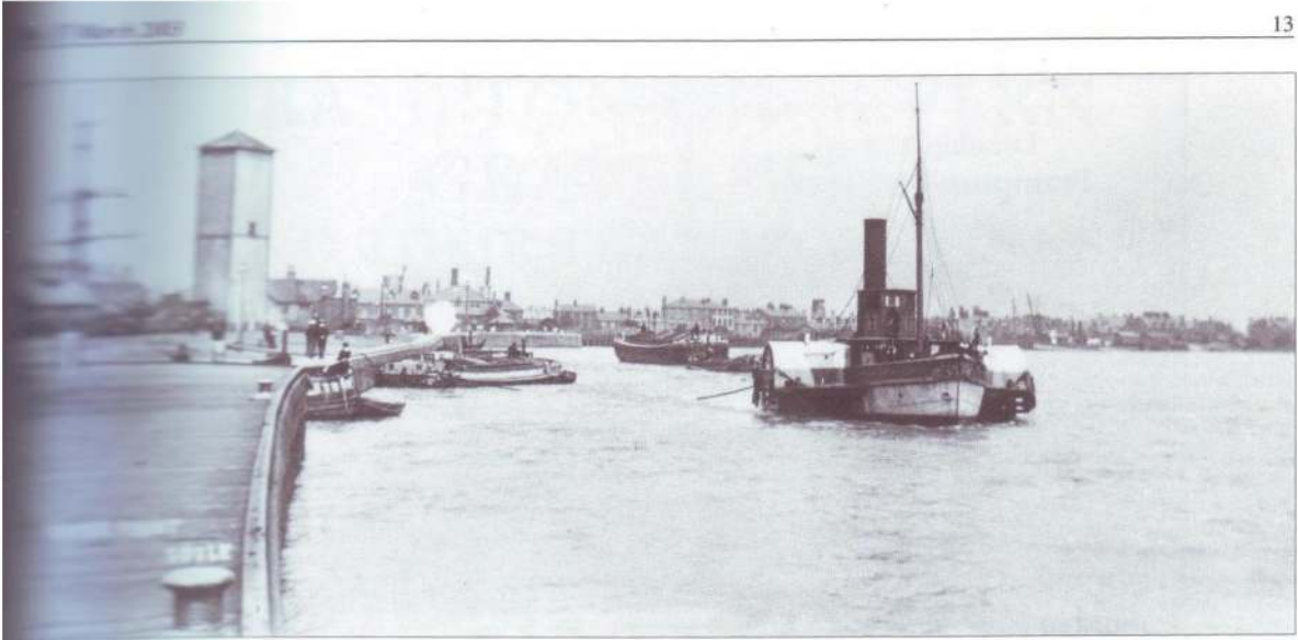
The Goole & Hull Steam Towing Company handled most inland waterway craft passing between the two ports as well as some coastal lighter traffic. Their paddle tug Shah is shown in the Ouse during the 1900s ready to tow barges downriver to Hull. The tug was built at South Shields and originally had two funnels side by side. A hydraulic accumulator tower may be seen and the stern of an inland waterway vessel visible as it prepares to enter Ship Lock and pen up into the docks. BM
