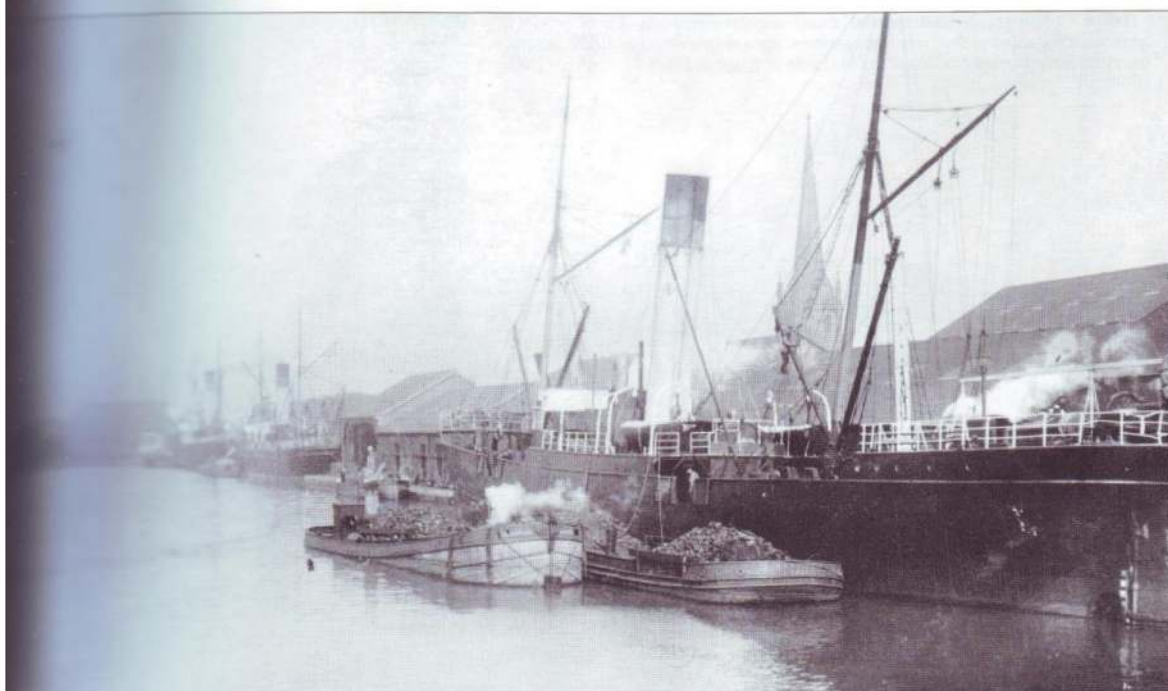
The 1100-ton steam keel West Riding , built by J. Scarr at Beverley in 1894, was purchased by Goole Steam Shipping Company in 1901 to supply coal, lubricants and water to their ships at Goole and is shown here moored alongside its lighter which is actually bunkering a ship in Railway Dock. West Riding followed the company through all its changes of ownership until it was sold in 1947. MT
